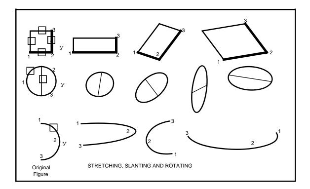
The illustrations above show how the same figure may be stretched, slanted, or rotated, depending on how the three points at the new position are placed.
